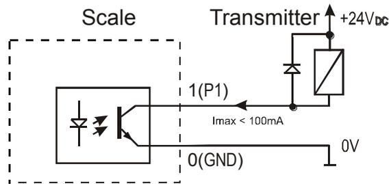
The outputs are adapted for direct connection of RM96P transmitter with DC24V input voltage and AC250V 8A output. The transmitter coil should be protected (shunt) with a diode, e.g. 1N4148.
