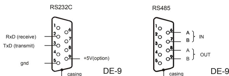
To connect the scale to the computer use RS232C connector delivered with the indicator.
