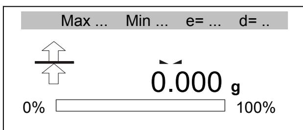
To read the mass, currently placed on the balance, use *X* key. Reuse of that key cause return to the maximum value.
