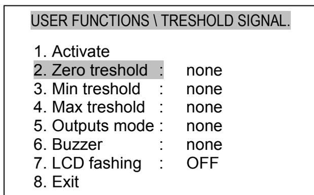
Using  $\vee$  and  $\wedge$  keys, move cursor to *Zero threshold* option and press *ENTER*.
