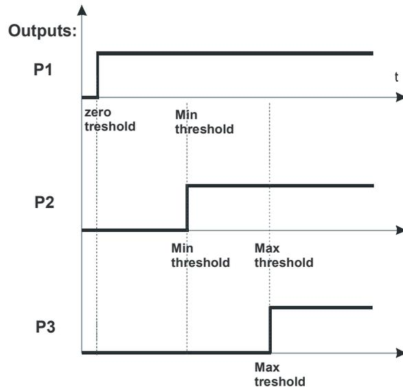
The *THRESHOLDS* connection contains three transistor outputs P1, P2 and P3 of open collector type, with load capacity 100mA/24V. The connected relays are not supplied from the balance and require additional 24V power supply unit. The relays inputs must be protected with diodes, e.g. 1N4148.
