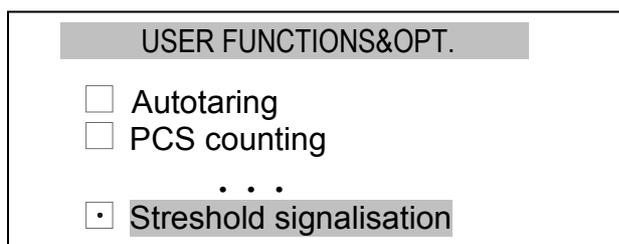
Press *MENU* key to enter the user functions menu, select *Threshold signalling* with cursor and press *ENTER*.
