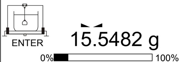
Suspend the plunger and immerse in beaker with examine liquid (measurement in the liquid) and press *ENTER*.
