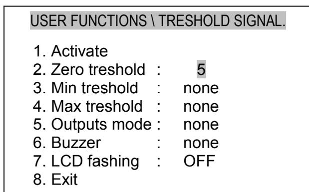
Enter the indications value, below which the balance is considered unloaded (no signalisation) and press *ENTER*.
