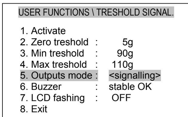
The *Outputs mode* option is used for setting the THRESHOLDS connection operation mode (see below). The appropriate mode is selected with  $<$  and  $>$  keys, confirmation – with *ENTER* key.
