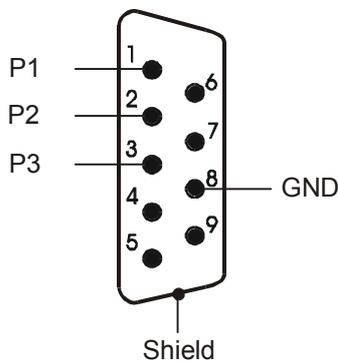
Scheme for connecting the single relay to *THRESHOLDS* connection output
