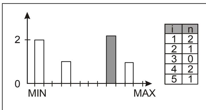
*F2* key prints the histogram. Table on the left shows division into subranges (*i*) and numbers of samples (*n*) in the individual subranges. Return to report displaying takes place after pressing *CLR* key.
