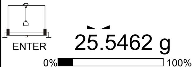
Suspend the plunger (measurement in the air) and press Enter. Please not immerse plunger in the liquid on this stage.
