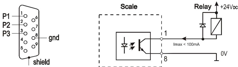
*Relays* output is the open collector transistor output with load capacity 100mA / 24V. Transmitter inputs must be protected with diodes, e.g. 1N4148. It is advised to use MS3K/P electronic board (sold separately), consisting of RM96P transmitters, with DC24V input voltage and AC250V, 3A output.
