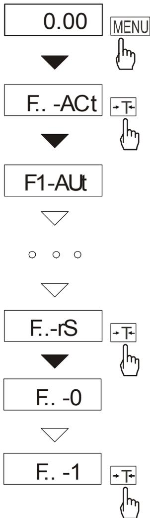
This function enables to select special functions that will be displayed after pressing *MENU* key. Easy access to the most useful functions will shorten operation time and make work more comfortable.
