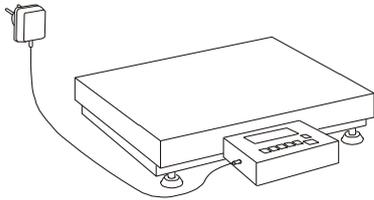
Leave the pan empty, plug the scale to the mains with a ground contact.
