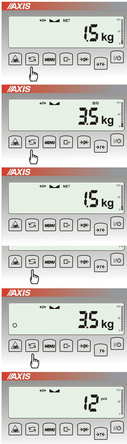
During standard weighing
