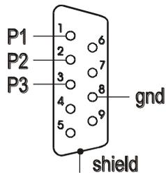
The Output connector is an optocoupler open collector output with a load capacity of 25mA / 24V. It is recommended to use ready-made MS 3K/P board, which contains RM96P relays with DC 24V input voltage and output: AC 250V, 3A.
