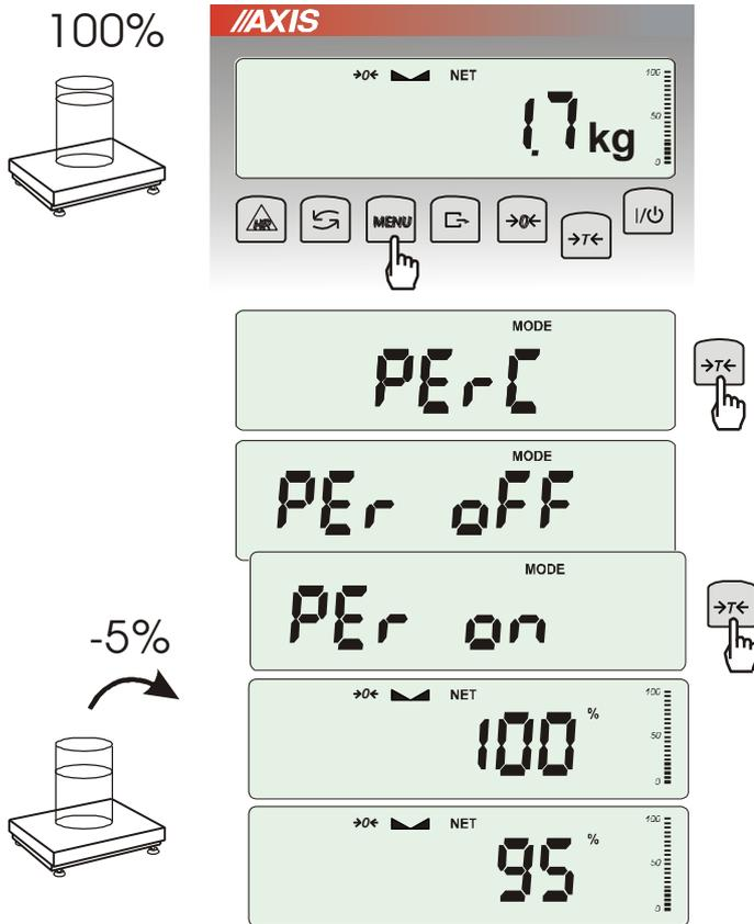
This function allows displaying weighing result in percents.
