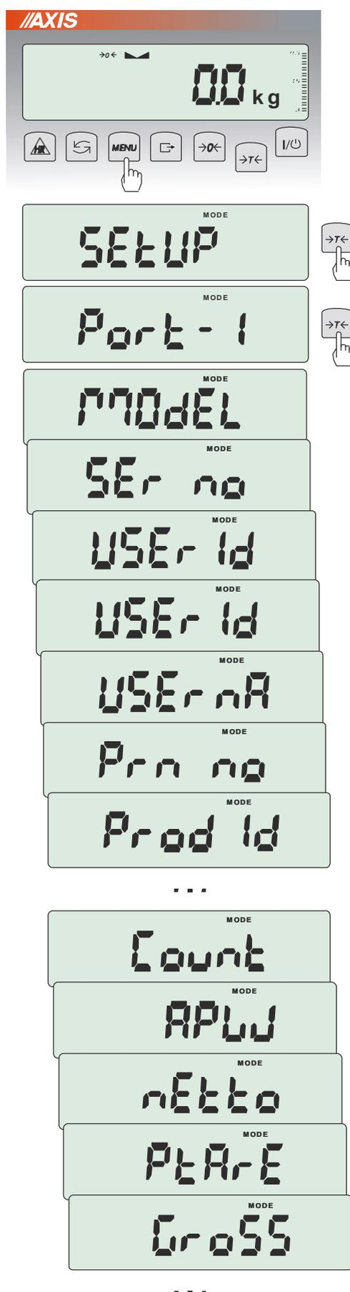
Function is used for printing additional information stored in scale memory, weighed product identification data and scale operator id. That information is inscribed using scale keys or scanner. After entering selected port (scale can have two ports) user may activate printout positions:
