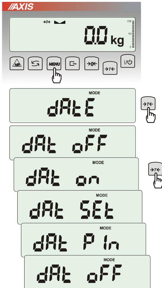
The function allows setting current date and time of scale internal clock and mode of its use.
