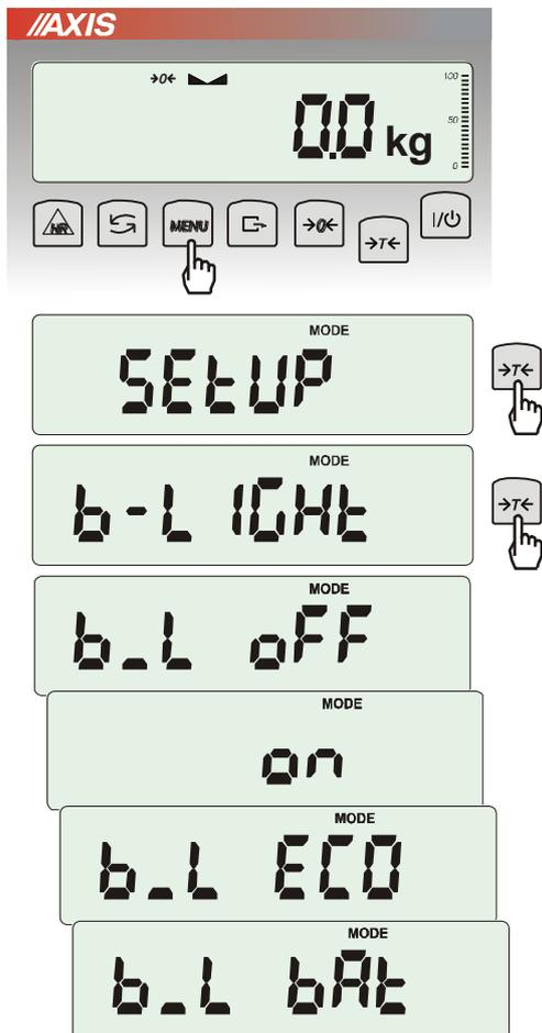
The function is used for choosing the work mode of scale display backlight:
