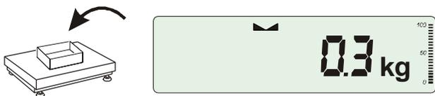
After putting container (package) tare the scale using  $\rightarrow T \leftarrow$  key. NET indicator will show up.
