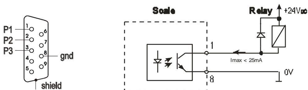
Relays output is the open collector transistor output with load capacity 25mA / 24V. Transmitter inputs must be protected with diodes, e.g. 1N4148.
