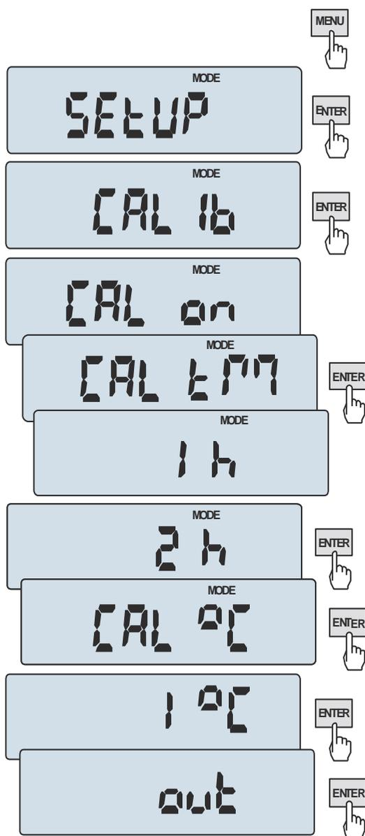
Press *MENU* key to display function menu and choose *CAL Ib* function by pressing *ENTER* key when it is displayed.
