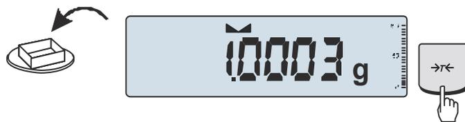
After putting container (package) tare the scale using  $\rightarrow T \leftarrow$  key.
