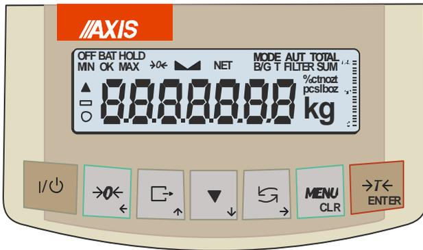
Scale display test (autotests of internal electronic elements C1:8 displayed only when any test result is negative)
