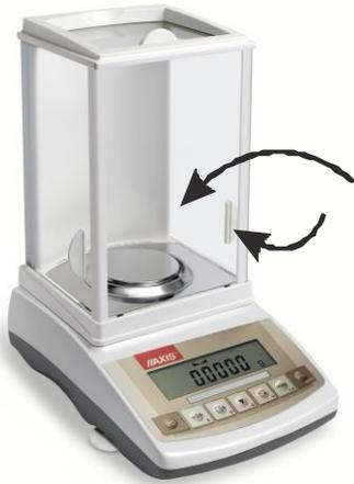
If the scale is not loaded and  $\rightarrow 0 \leftarrow$  indicator doesn't indicate, press  $\rightarrow 0 \leftarrow$  key.
