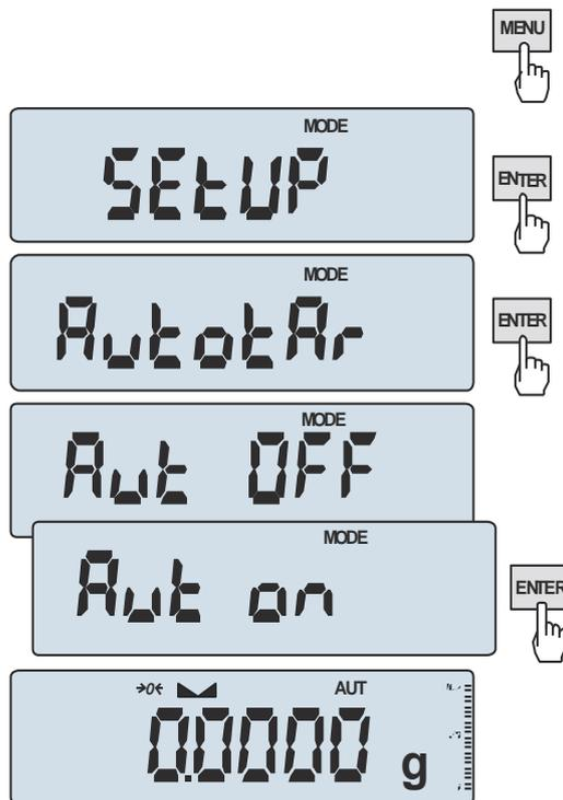
When the function is activated, the scale automatically ensures stable zero indication if the pan is empty or if zero indication was acquired by pressing *ENTER* key.
