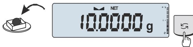
In order to readout gross weight press  $\rightarrow \curvearrowright \leftarrow$  key (B/G indicator shows that scale indicates gross weight). Press again  $\rightarrow \curvearrowright \leftarrow$  key in order to come back to net indications.
