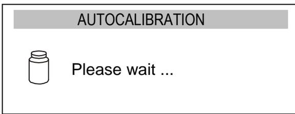
Afterwards the balance enters automatically into internal calibration mode, which is described with details in next chapter. Calibration can be terminated using *CLR* key.
