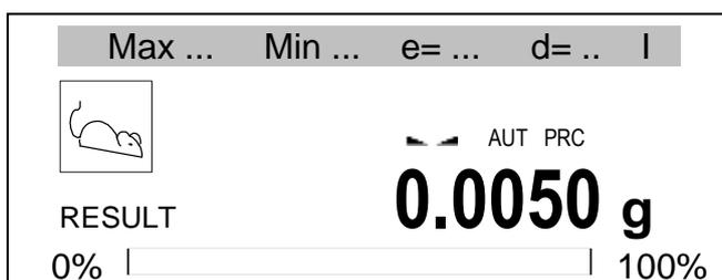
The balance makes a series of measurements and displays result. After unloading the balance is ready for next measurement. The balance will show stable (averaged) result and will send it through serial port. To end working with the function press *MENU* key, choose *Animal* and *Deactivation*.
