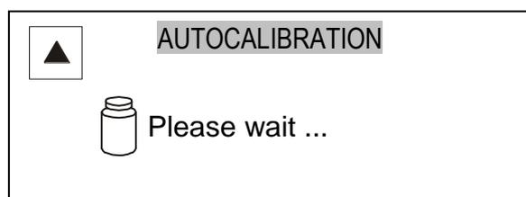
When internal calibration is performed successfully the balance indicates zero on the display at empty pan.
