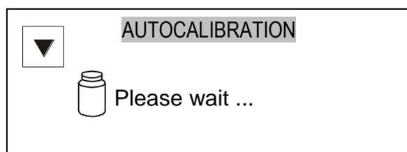
During calibration internal weight is put three times on and obtained results are compared.
