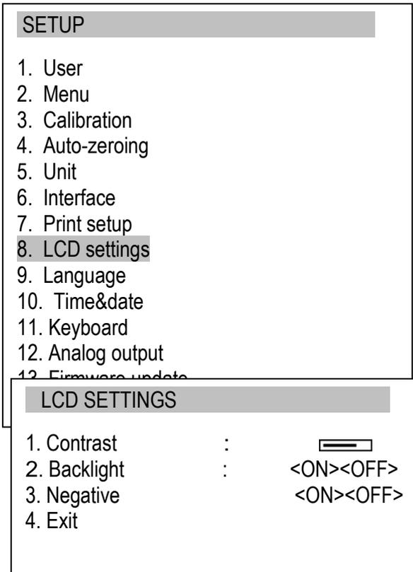
LCD settings enable to set contrast and backlight.
