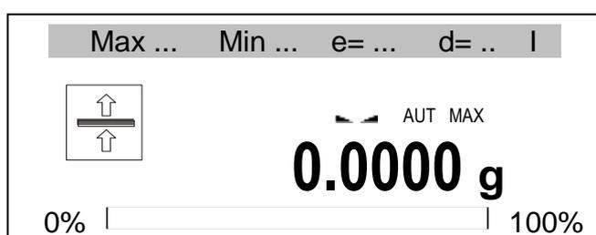
→T← key causes balance zeroing and enables to start next series of weighing.
