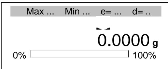
When internal calibration is finished, the balance enters into normal weighing mode.
