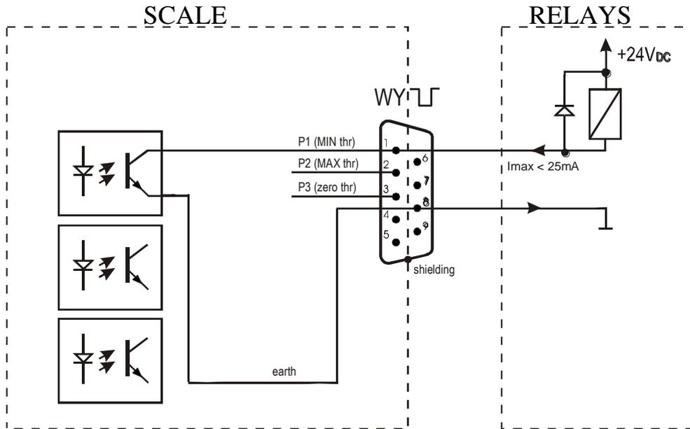
Relays output is the open collector transistor output with load capacity 25mA / 24V. Transmitter inputs must be protected with diodes, e.g. 1N4148.
