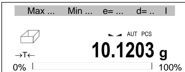
Put empty container on pan and press →T← key.
