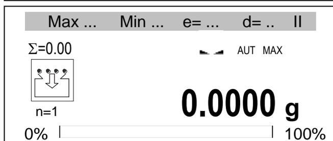
The balance is ready for weighing the successive ingredients, and after each ingredient it is necessary to press  $\rightarrow T \leftarrow$  key. It will zero the balance indications. On the left side the sum of previously weighed ingredients ( $\Sigma$ ) and their number (n) is displayed.
