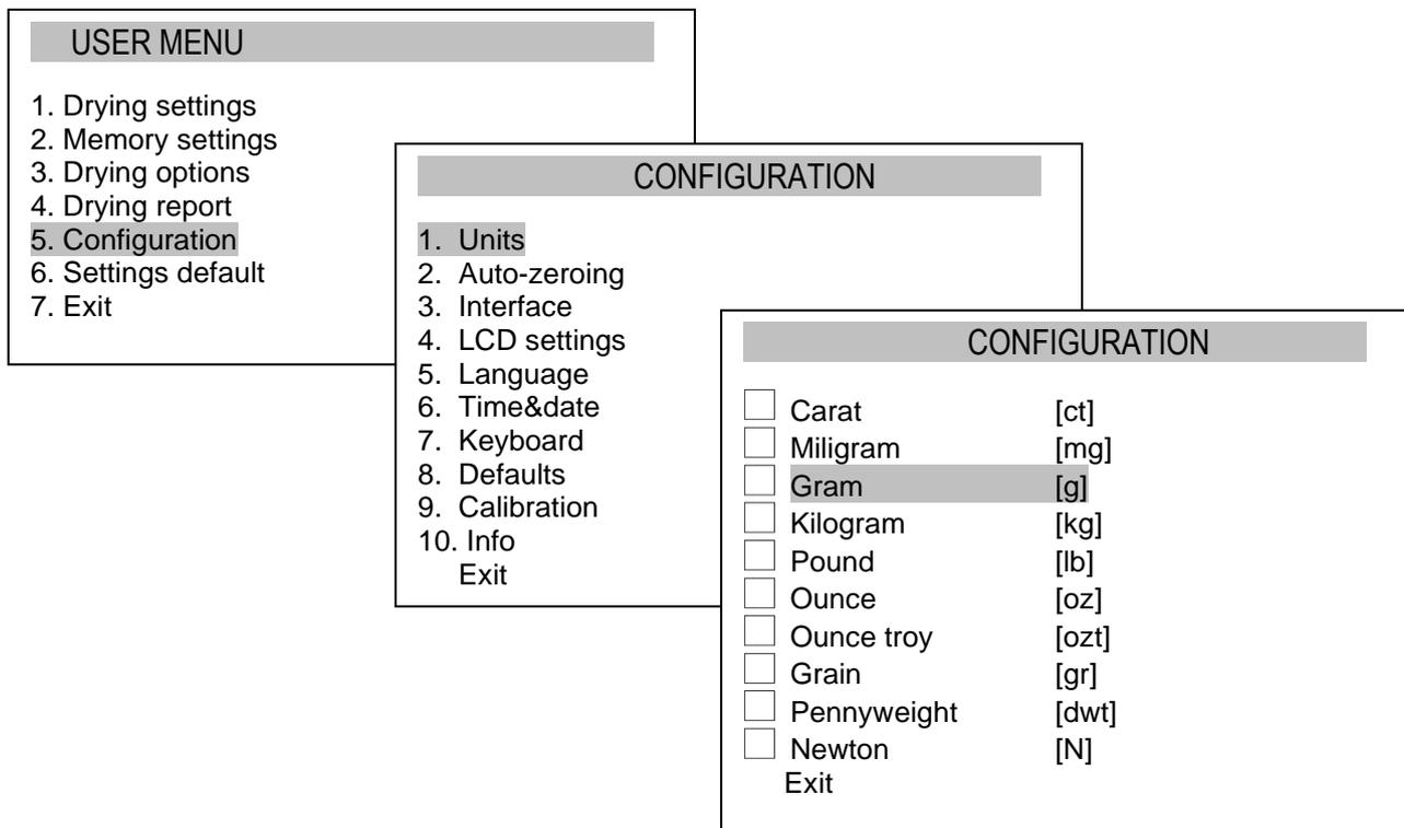
Choice of unit is made using navigation keys and ENTER key.
