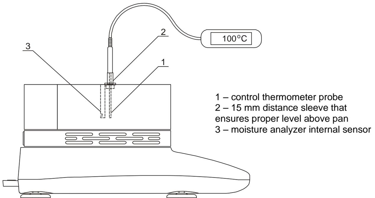
Before executing temperature correction (inscribing T1 and T2 temperature) drying cycle must be made with inscribed T1 temperature and drying time 15 minutes. Single-use pan (a new one) should be put on the pan. When drying process is almost done write down moisture analyzer temperature indication (T value on the left side of moisture analyzer display) and control thermometer indications. Both indications are needed for correction:
