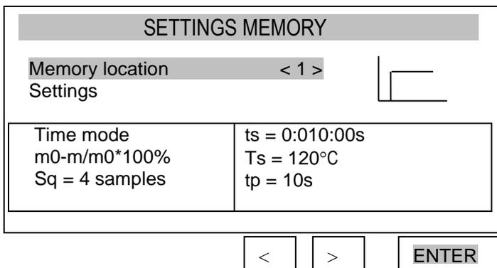
Select a number of desired settings using navigation keys < and >. Press *ENTER* to accept.
