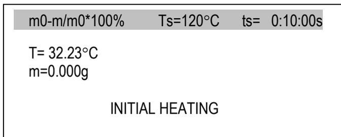
Initial heating should warm the drying chamber up to 105°C within 3 minutes. When temperature during initial heating exceeds 105°C or heating time is longer than 3 minutes, terminate initial heating with CLR key and check if the analyser is not damaged (see chapter 15).
