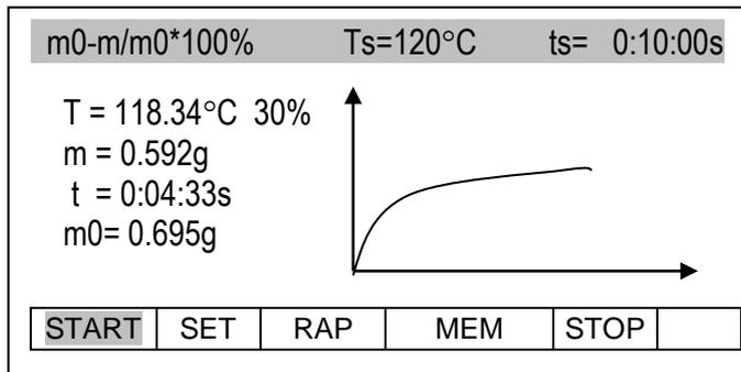
When drying chart is visible, place a sample on the pan and choose *START* option (*F1* key). Drying parameters and drying process chart are presented on the display.
