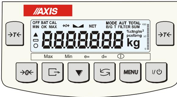
Scale display test (autotests of internal electronic elements C1:8 displayed only when any test result is negative)
