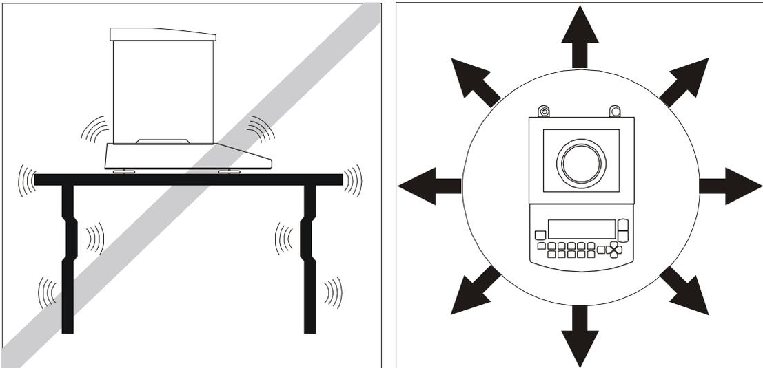
Location for the balance should be chosen with care in order to limit influence of the factors that can interrupt working balance. This location has to maintain proper temperature for working balance and necessary space for its operating. The balance should stay on stable table made of material that does not influence magnetically on the balance.
