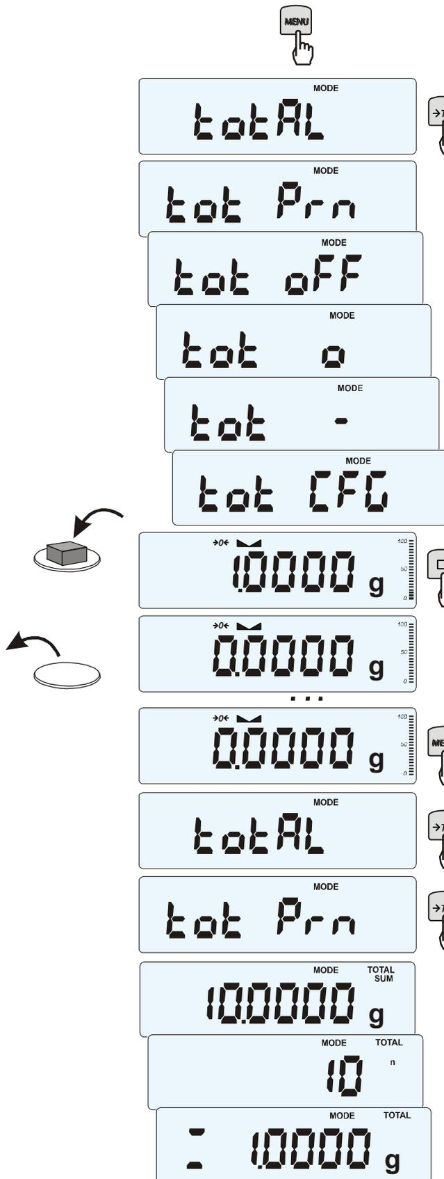
The function allows calculating total weight for series of measurements, which can be greater than scale capacity. It allows calculating total weight as well as average value.
