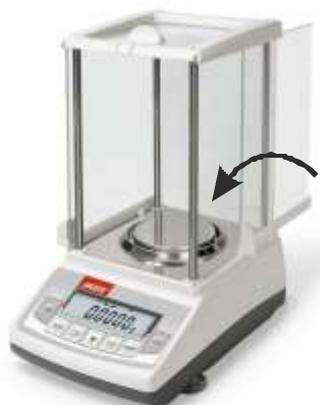
Balance indication should be readout when the weighing chamber is closed and the result is stable.
