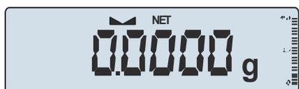
Put on weighted object and readout net weight (NET indicator shows that scale indicates net weight).
