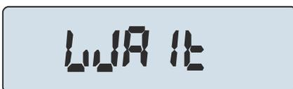
Internal calibration – about 1 minute (press ▼ key if You want to terminate calibration)
