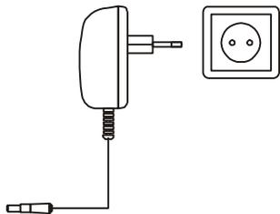
Plug feeder into ~230V power supply socket. When the pan is empty plug feeder output connector into 12V socket at back of the scale. Autotests and internal calibration will be performed.
