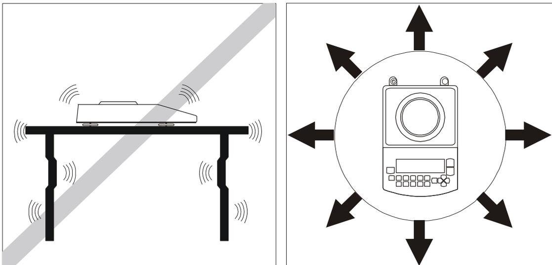
Location for the scale should be chosen with care in order to limit influence of the factors that can interrupt working scale. This location has to maintain proper temperature for working scale and necessary space for its operating. The scale should stay on stable table made of material that does not influence magnetically on the scale.
