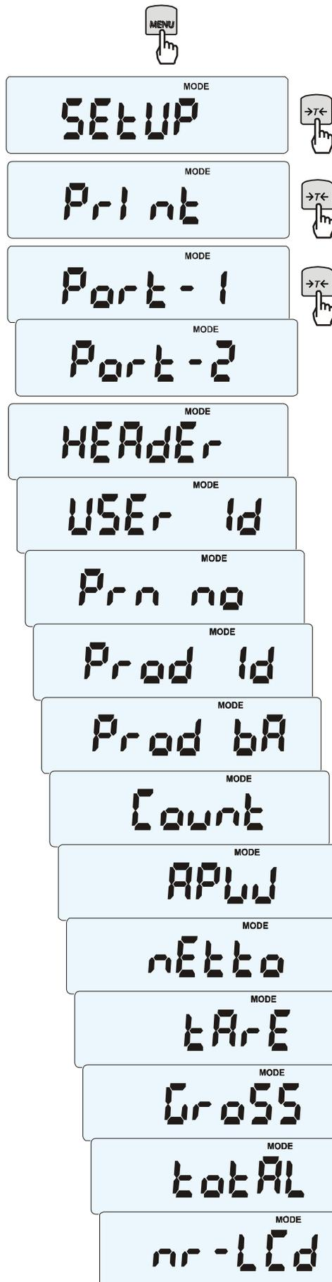
Function is used for printing additional information stored in scale memory, weighed product identification data and scale operator id. That information is inscribed using scale keys or scanner.
