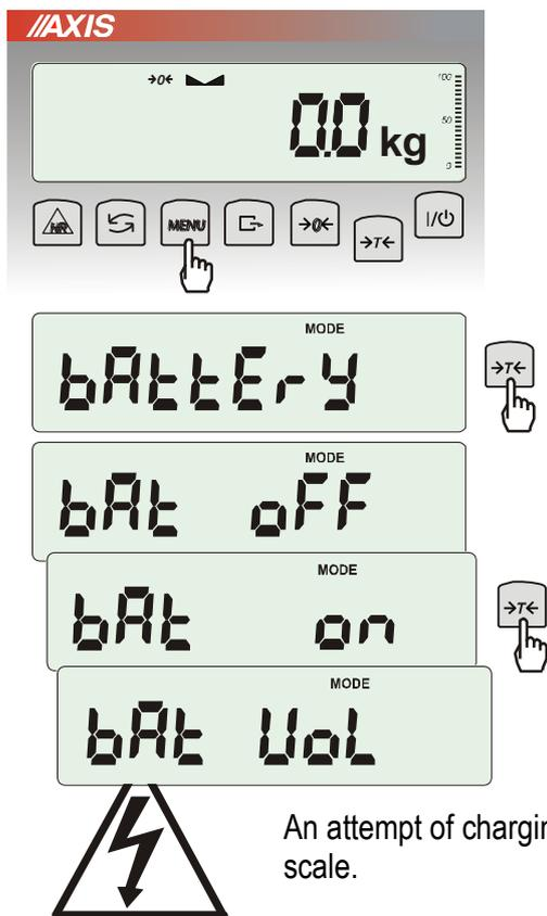
An attempt of charging ordinary batteries can cause serious damage of the scale.
