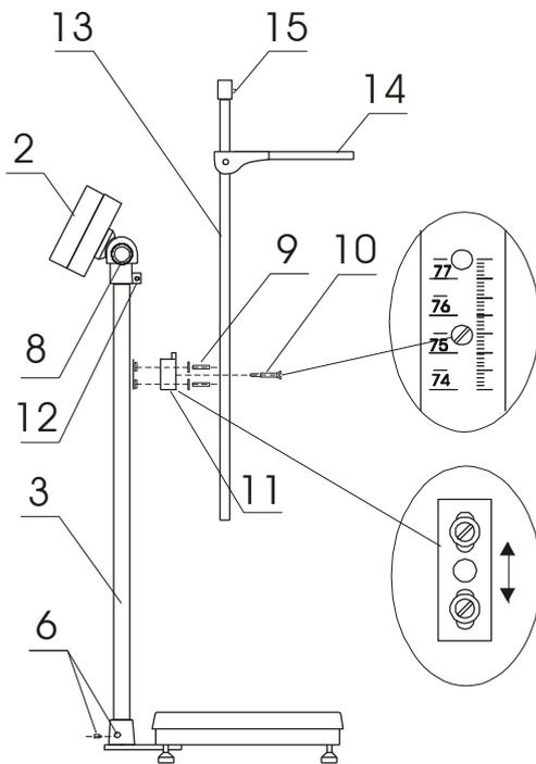
1. Loosing screw 12 turn indicator 2 in the direction of person operating the scale.
