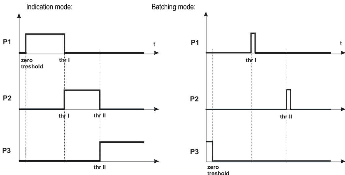
In *Batching mode* on P1 (thr I) and P2 (thr II) outputs short-circuit impulses appears for time of 0,5s. On P3 (zero) output short-circuit state appears when indication does not exceed threshold value signalling zero load.
