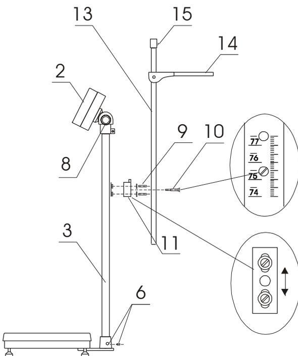
1. Loosing handwheel 8 set indicator 2 in suitable position.
