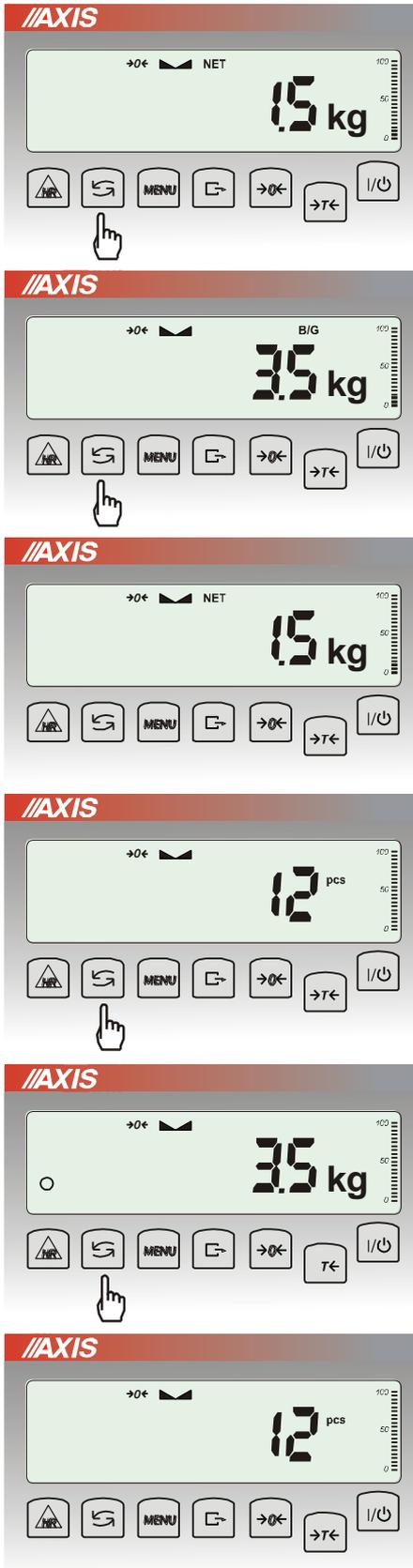
During standard weighing
