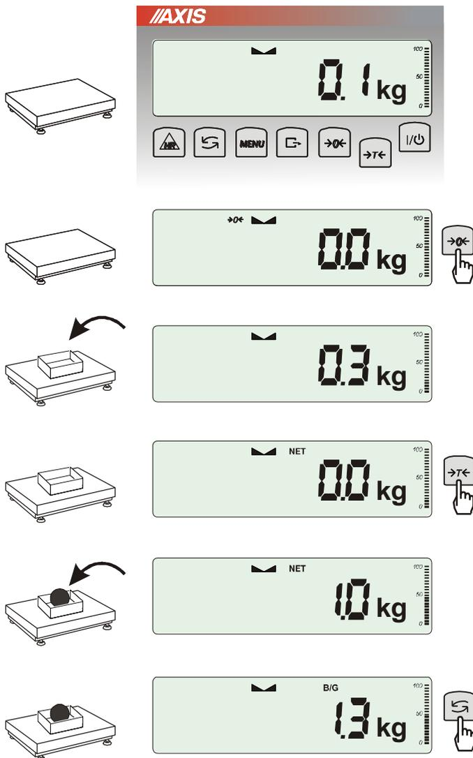
If the scale is not loaded and →0← indicator doesn't indicate, press →0← key.
