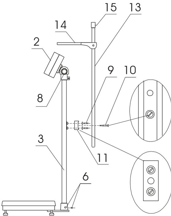
1. Loosing handwheel 8 set indicator 2 in suitable position. Using the pair of screwed sockets located lower on the column 3, screw distance cube 11 with screws 9.
