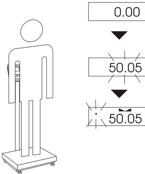
Switching power supply of the scale on, causes special function of person weighing (LOC) is automatically started.
