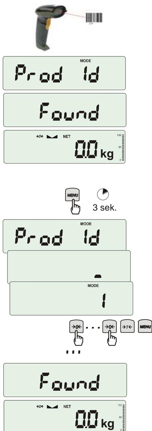
The fastest way to recall product from database is to readout his barcode number (*Prod bA*) by using barcode reader (option). It can be done in any moment.
