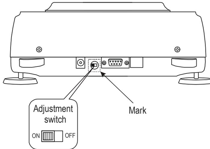
Performing calibration requires changing adjustment switch position, which is placed behind protecting mark (sticker) of a notified body. An access to the switch is possible only after removing the mark. Therefore, scale calibration causes lost of legal verification and, in consequence, the necessity of renew legal verification in the nearest notified body or in place where the balance is used.
