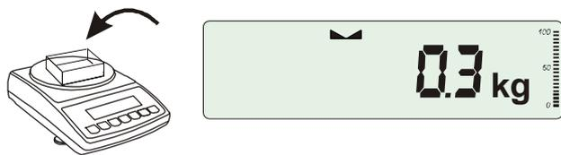
After putting container (package) tare the scale using  $\rightarrow T \leftarrow$  key. NET indicator will show up.
