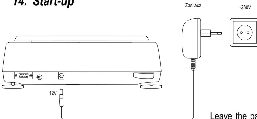
Leave the pan empty, plug the scale to the mains with a ground contact.
