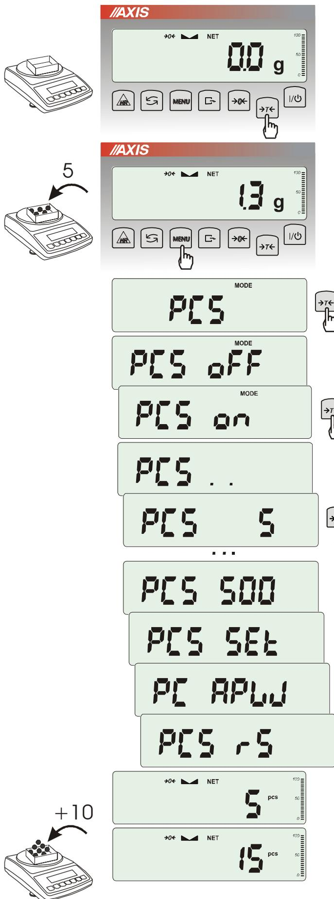
This function enables to count identical pieces, e.g. turnbuckles or buttons.
