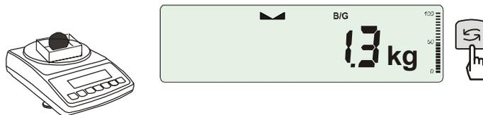
In order to readout gross weight press  $\rightarrow \text{G} \leftarrow$  key (B/G indicator shows that scale indicates gross weight). Press again  $\rightarrow \text{G} \leftarrow$  key in order to come back to net indications.
