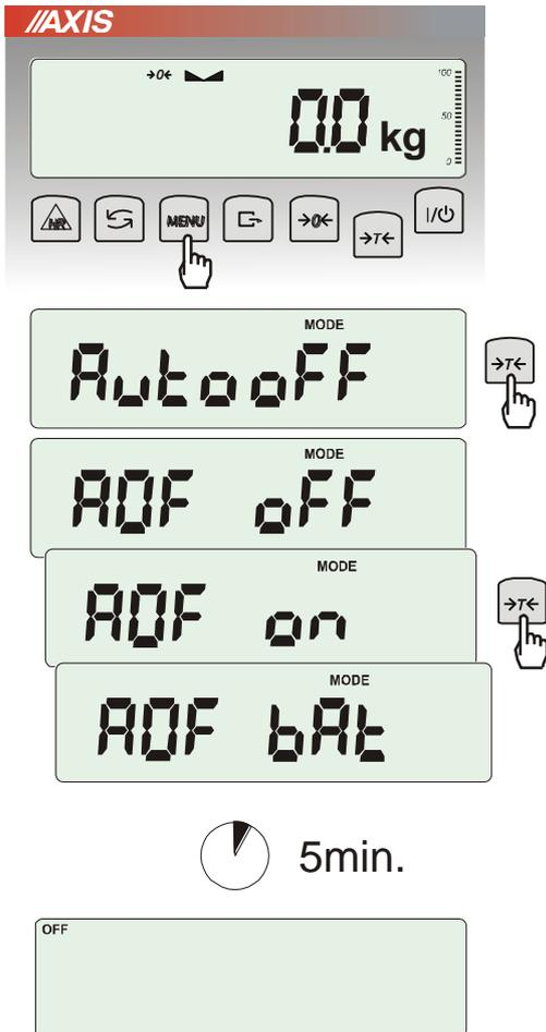
The function is helpful in scales supplied from accumulators. The function causes scale to switch off automatically.
