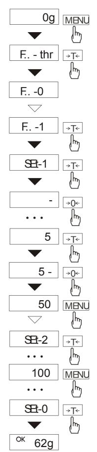
This function compares weighing result with two reference values: lower and upper threshold. The balance signalises comparison result with MIN, OK and MAX indicators and sound signal generated when threshold values are exceeded.
