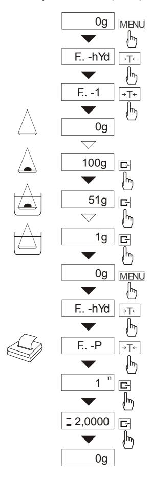
This function calculates material density basing on its weight in air and in liquid of known density using the formula below:
