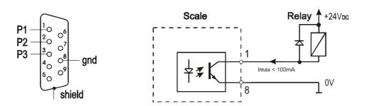
*PROGI* output is the open collector transoptor output with load capacity 100mA / 24V. Transmitter inputs must be protected with diodes, e.g. 1N4148.
