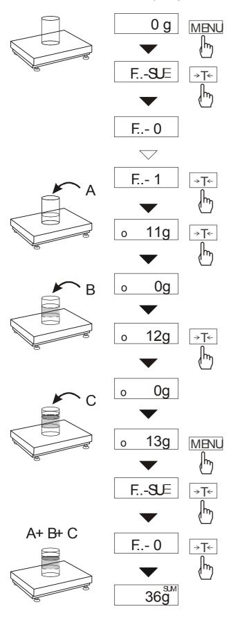
This function allows separate weighing of several ingredients in one container with a possibility to control aggregated sum of all weighed components.
