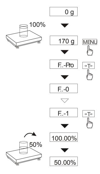
This function enables to display weighing result as a percentage of a reference sample.
