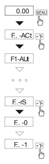
This function enables to select special functions that will be displayed after pressing *MENU* key. Easy access to the most useful functions will shorten operation time and make work more comfortable.
