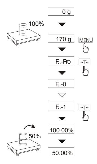
This function enables to display weighing result as a percentage of a reference sample.
