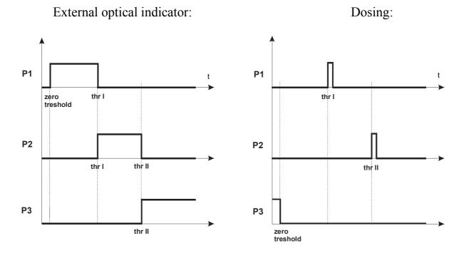
During dosing (optional), short-circuit pulses lasting for 0.5s appear on P1 (I threshold) and P2 (II threshold) outputs and for P3 output (zero threshold) – short-circuit state for the indication below zero threshold.
