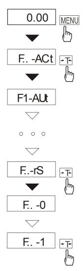
This function enables to select special functions that will be displayed after pressing *MENU* key. Easy access to the most useful functions will shorten operation time and make work more comfortable.
