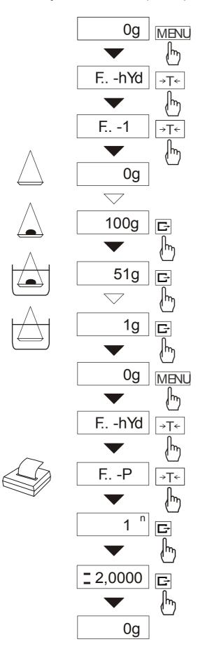
This function calculates material density basing on its weight in air and in liquid of known density using the formula below:
