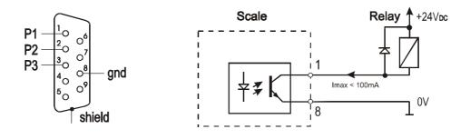
*Relays* output is the open collector transoptor output with load capacity 100mA / 24V. Transmitter inputs must be protected with diodes, e.g. 1N4148. It is advised to use MS3K/P electronic board (sold separately), consisting of RM96P transmitters, with DC24V input voltage and AC250V, 3A output.
