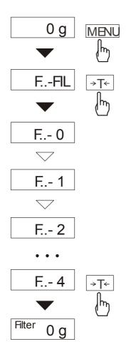
This function activates digital filter of chosen intensity, which reduces the influence of mechanical vibrations (air blasts, base vibrations) on measurement result. Using the filter is necessary for accurate people or animal weighing.
