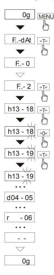
This function enables to set current date and time of internal balance clock and enable/disable date and time on weighing result printouts.
