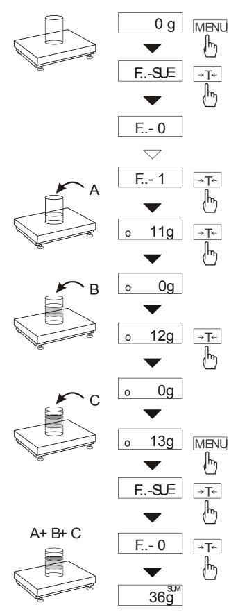
This function allows separate weighing of several ingredients in one container with a possibility to control aggregated sum of all weighed components. Function options:
