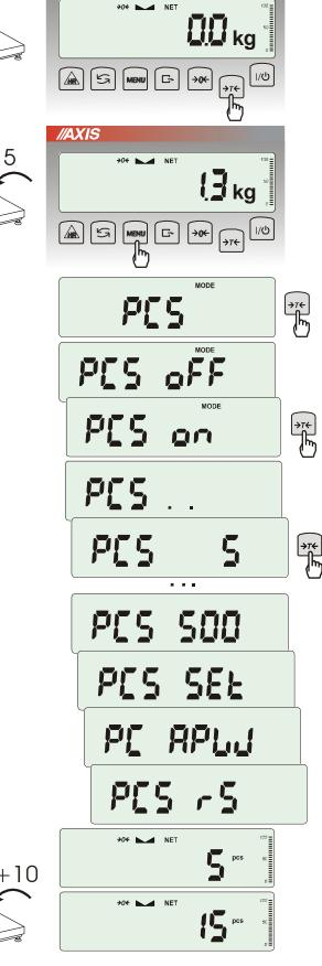
This function enables to count identical pieces, e.g. turnbuckles or buttons.
