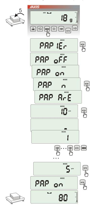
This function enables to calculate paperweight of  $1m^2$  of paper basing on samples of known area. For quick access, the function is accessible directly by pressing *MENU* key.
