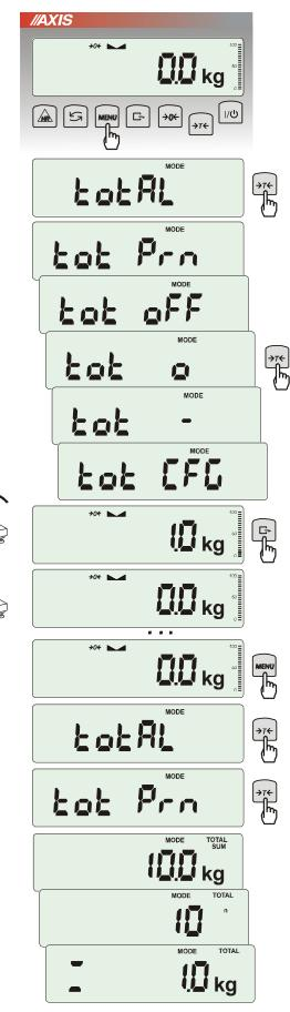
The function allows calculating total weight for series of measurements, which can be greater than scale capacity. It allows calculating total weight as well as average value.
