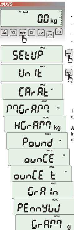
The function allows selecting weighing unit:
