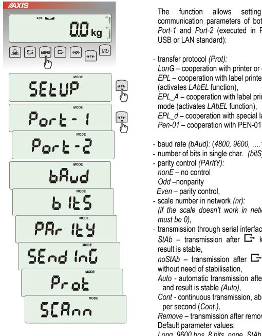
communication parameters of both of serial ports Port-1 and Port-2 (executed in RS232C, RS485,
