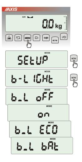
The function is used for choosing the work mode of scale display backlight:
