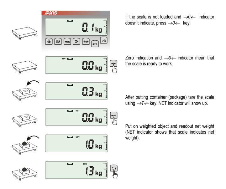
In order to readout gross weight press P key (B/G indicator shows that scale indicates gross weight). Press again P key in order to come back to net indications.
