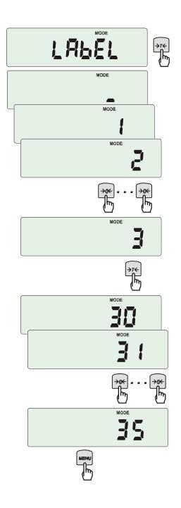
Press *MENU* button. When *LAbEL* is displayed press  $\rightarrow T \leftarrow$  key. Actual label number will show. To enter new label number press  $\rightarrow T \leftarrow$  key, to exit function without number change press *MENU*.
