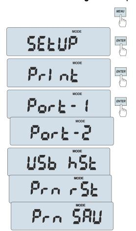
The option allows you to obtain extended printouts after pressing the key for a long time —. The printouts additionally contain information identifying the weighed product and the scale user, previously saved in memory using the scale or scanner keys.
