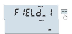
Selecting the FIELd \_ ... option opens the process of filling ir the print field using the scale's navigation  $\leftarrow$  keys ,  $\uparrow$  ,
