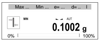
Load under MIN threshold.
