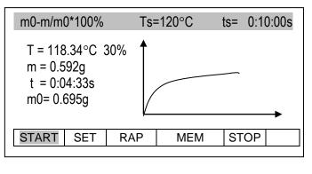
When drying chart is visible, place a sample on the pan and choose *START* option (*F1* key). Drying parameters and drying process chart are presented on the display.
