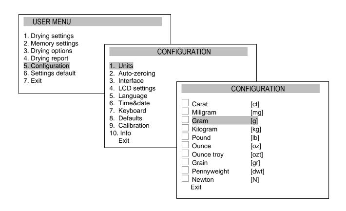
Choice of unit is made using navigation keys and ENTER key.
