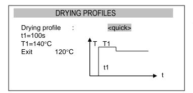
*Drying profile* will be used to optimization of drying process by accommodation a process to physical properties of sample material.
