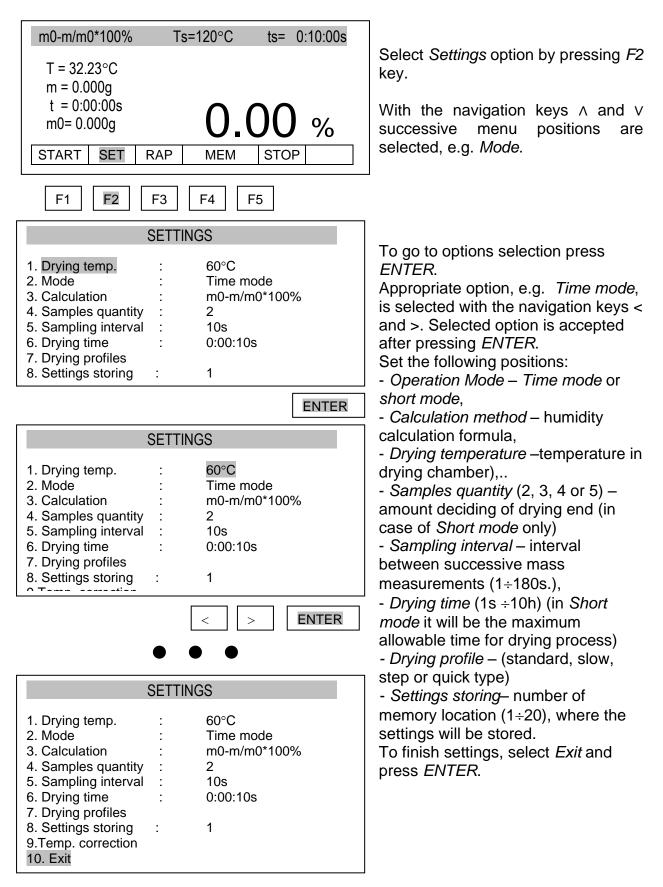
*Note:* All defined parameters are stored in the memory until the next changed (also after unplugging the device from the mains).
