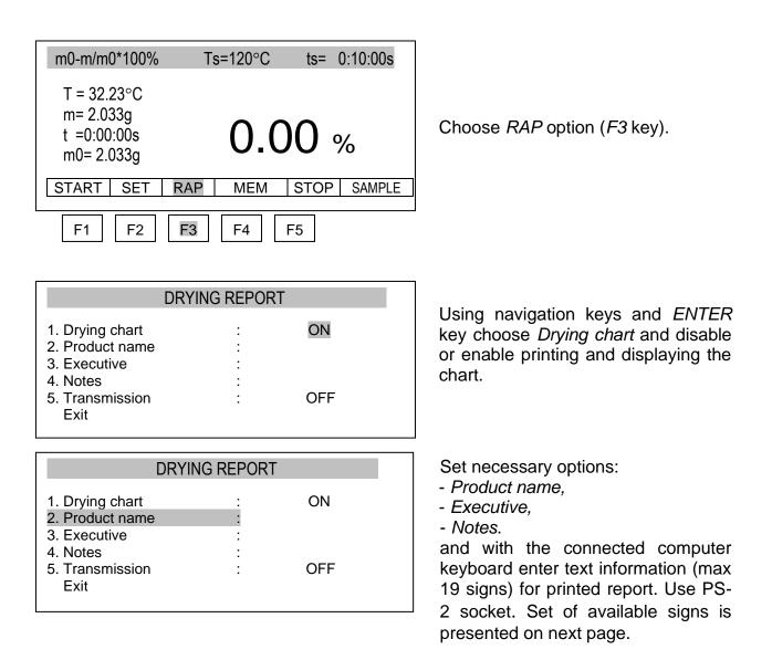
Activation of *Transmision* option will activate sending of all sampling results through the RS232C port. The may be printed by the printer or stored in the computer, e.g. by the *Promas* software.
