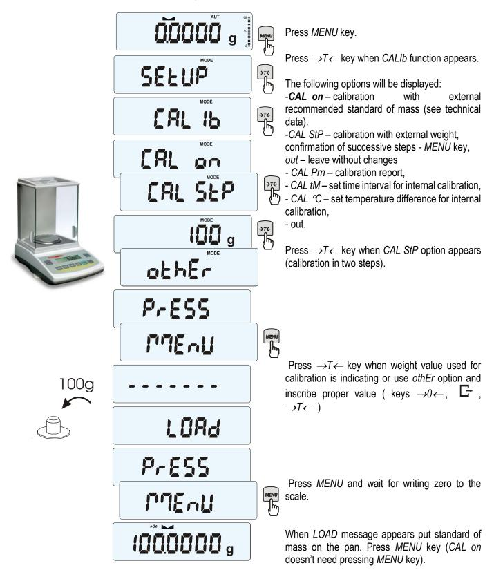
Wait until internal calibration is finished and zero indication is displayed.
