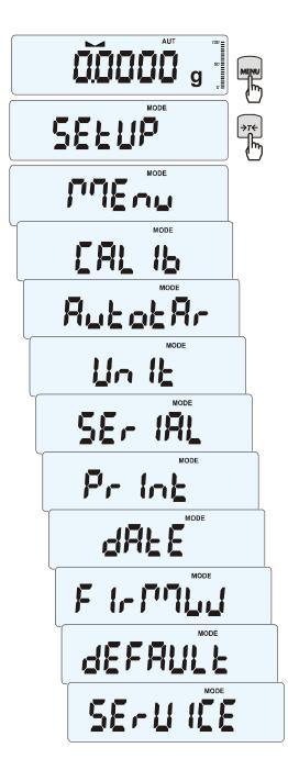
*SEtUP* contains all options used for setting scale work mode:
