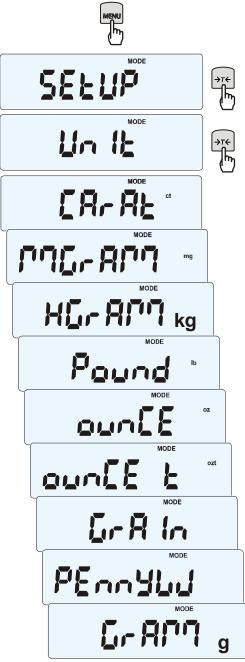
The function allows selecting weighing unit:
