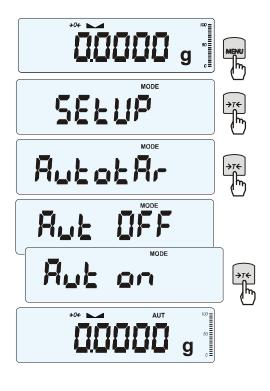
When the function is activated, the scale automatically ensures stable zero indication if the pan is empty or if zero indication was acquired by pressing  $\rightarrow T \leftarrow$  key.
