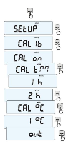
Press *MENU* key to display function menu and choose *CALIb* function by pressing  $\rightarrow T \leftarrow$  key when it is displayed.
