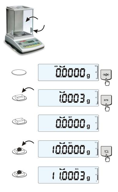
If the scale is not loaded and  $\rightarrow 0 \leftarrow$ indicator doesn't indicate, press  $\rightarrow 0 \leftarrow$  key.
