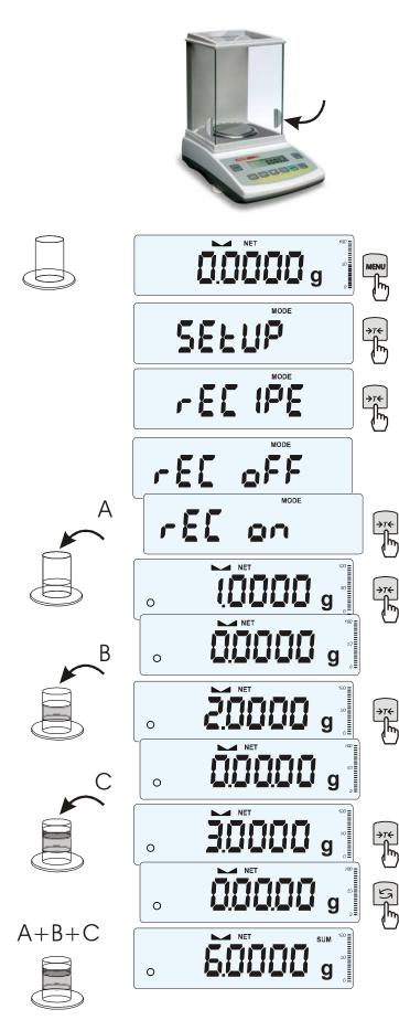
The function allows for separate weighing of several ingredients in one container with the possibility of reading current sum of all weighed ingredients.
