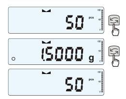
When special function e.g. *PCS* is turned on, using  $\uparrow$  key enables to go back to standard weighing mode.
