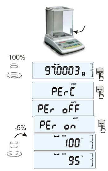
This function allows displaying weighing result in percents.
