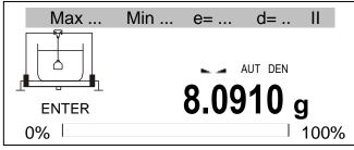
Hang plunger in liquid – measurement in liquid – and press *ENTER*.
