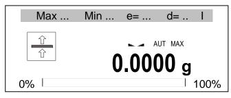
→T← key causes balance zeroing and enables to start next series of weighing.
