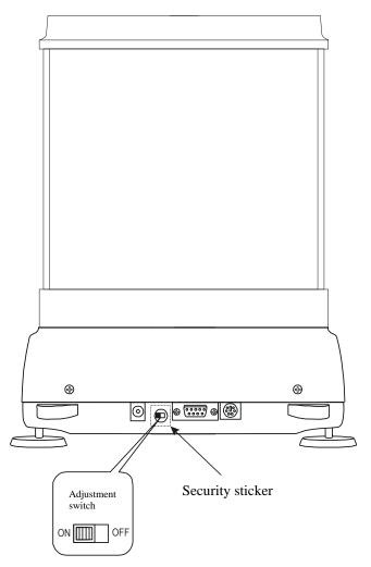
In balances comply with verification requirements performing calibration requires changing adjustment switch position, which is placed behind protecting mark (sticker) of a notified body. An access to the switch is possible only after removing the mark.
