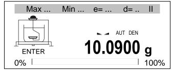
Put material on upper pan (measurement in air) and press *ENTER*.
