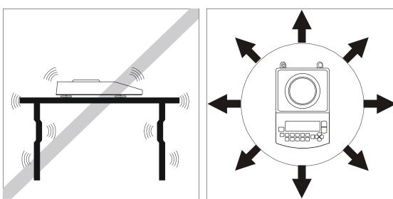
Location for the balance should be chosen with care in order to limit influence of the factors that can interrupt working balance. This location has to maintain proper temperature for working balance and necessary space for its operating. The balance should stay on stable table made of material that does not influence magnetically on the balance.
