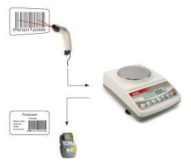
After selecting product it is possible to send (to computer or printer) actual indication with additional data, selected by *Print setup* option.
