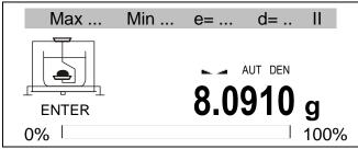
Put material on lower pan (measurement in liquid) and press *ENTER*.
