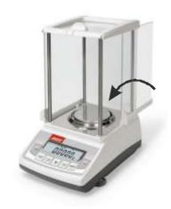
Balance indication should be readout when the weighing chamber is closed and the result is stable.
