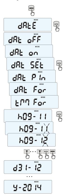
The function allows setting current date and time of scale internal clock and mode of its use.
