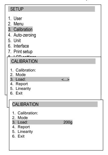
Load option enables inscribing standard of mass value, which will be used to calibrate (it is suggested to use standard of mass value close to balance's max).
