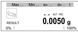
The balance makes a series of measurements and displays result. After unloading the balance is ready for next measurement.
