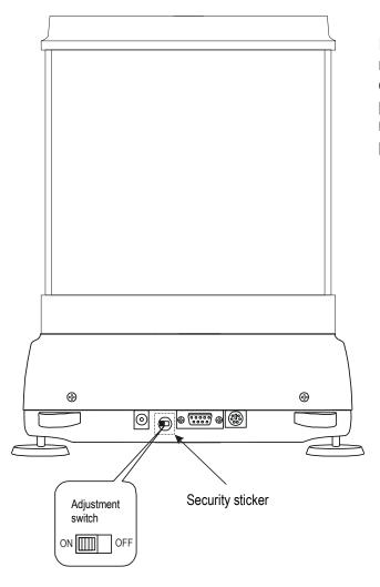
In balances comply with verification requirements performing calibration requires changing adjustment switch position, which is placed behind protecting mark (sticker) of a notified body. An access to the switch is possible only after removing the mark.
