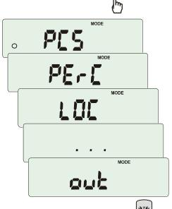
After adding all necessary functions press *out* in order to come back to weighing mode. User now after pressing *MEnu* key has access to selected earlier functions and to *SEtuP* option. *dEFAULt* option is used to set factory settings.
