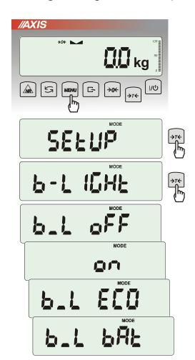
The function is used for choosing the work mode of scale display backlight:
