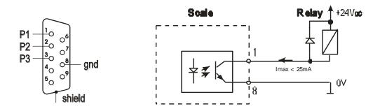
Relays output is the open collector transoptor output with load capacity 25mA / 24V. Transmitter inputs must be protected with diodes, e.g. 1N4148.
