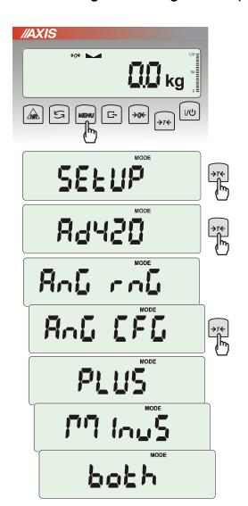
This option enables to set-up analog out (4-20mA or 0-10V) working method used e.g. in PLC regulators:
