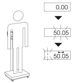
Switching power supply of the scale on, causes special function of person weighing (LOC) is automatically started.
