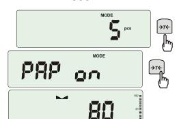
This function enables to calculate paperweight of  $1m^2$  of paper basing on samples of known area. For quick access, the function is accessible directly by pressing MENU key.
