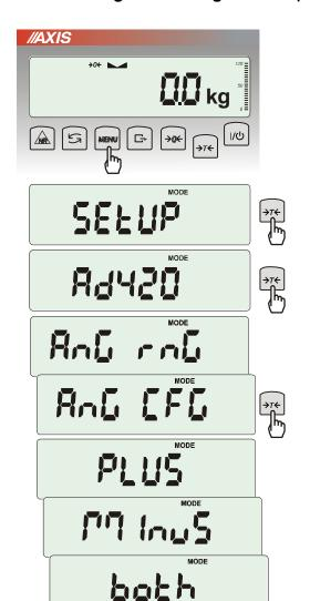
This option enables to set-up analog out (4-20mA or 0-10V) working method used e.g. in PLC regulators:
