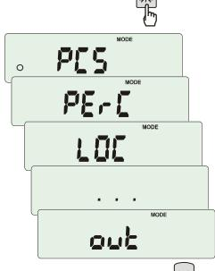
After adding all necessary functions press *out* in order to come back to weighing mode. User now after pressing *MEnu* key has access to selected earlier functions and to *SEtuP* option. *dEFAULt* option is used to set factory settings.
