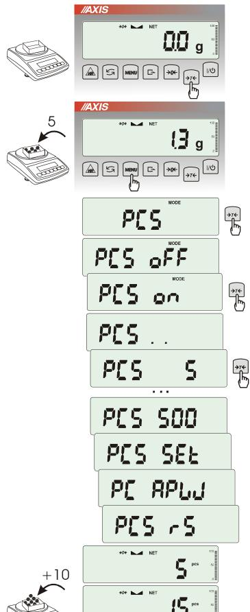
This function enables to count identical pieces, e.g. turnbuckles or buttons.
