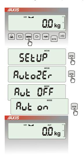
When the function is activated, the scale automatically ensures stable zero indication if the pan is empty or if zero indication was acquired by pressing  $\rightarrow T \leftarrow$  key.
