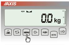
The function allows selecting weighing unit:
