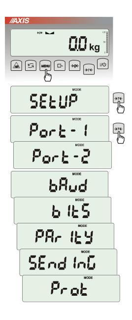
The function allows setting independently communication parameters of both of serial ports *Port-1* and *Port-2* (executed in RS232C, RS485, USB or LAN standard):
