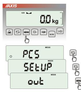
Accelerated working with menu: Menu first position is displayed for about 7s. During this time user can view next positions by using  $t \rightarrow key$  (or  $\rightarrow 0 \leftarrow$ ).
