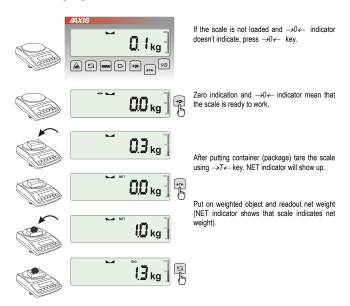
In order to readout gross weight press  $\mathfrak{P}$  key (B/G indicator shows that scale indicates gross weight). Press again  $\mathfrak{P}$  key in order to come back to net indications.
