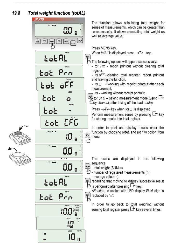
To leave the function with clearing total register, select *totAL* function from menu and choose *tot oFF* option. Scale prints the communicate informing about clearing registers.
