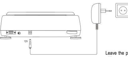
Leave the pan empty, plug the scale to the mains with a ground contact.
